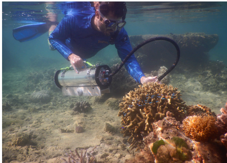
On the cover: Dr. Kenneth Hoadley uses the submersible algal phenotyping, or SAP, fluorometer to collect data on the health of a coral reef.
